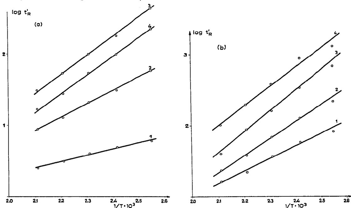
Fig. 1.  $\log t_R'$  versus  $1/T$  plots for the system  $\text{H}_2\text{O}$  (1)– $\text{EtOH}$  (2)– $\text{EtOAc}$  (3)– $\text{AcOH}$  (4) on 2 m × 0.4 cm columns of (a) Porapak Q and (b) Porapak T. Carrier gas (hydrogen) flow-rate, 150 ml/min.
