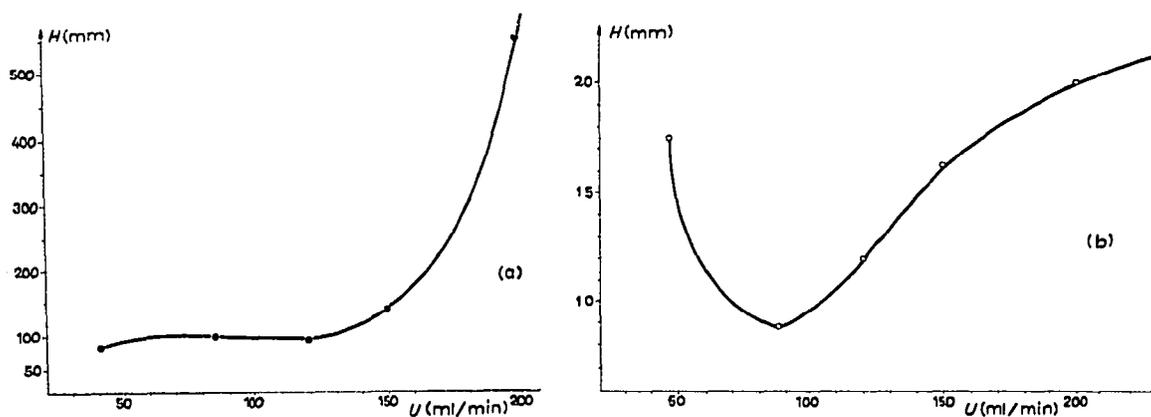
Fig. 2. Van Deemter plots of (a) methanol on Porapak Q and (b) ethanol on Porapak T at 120°.
