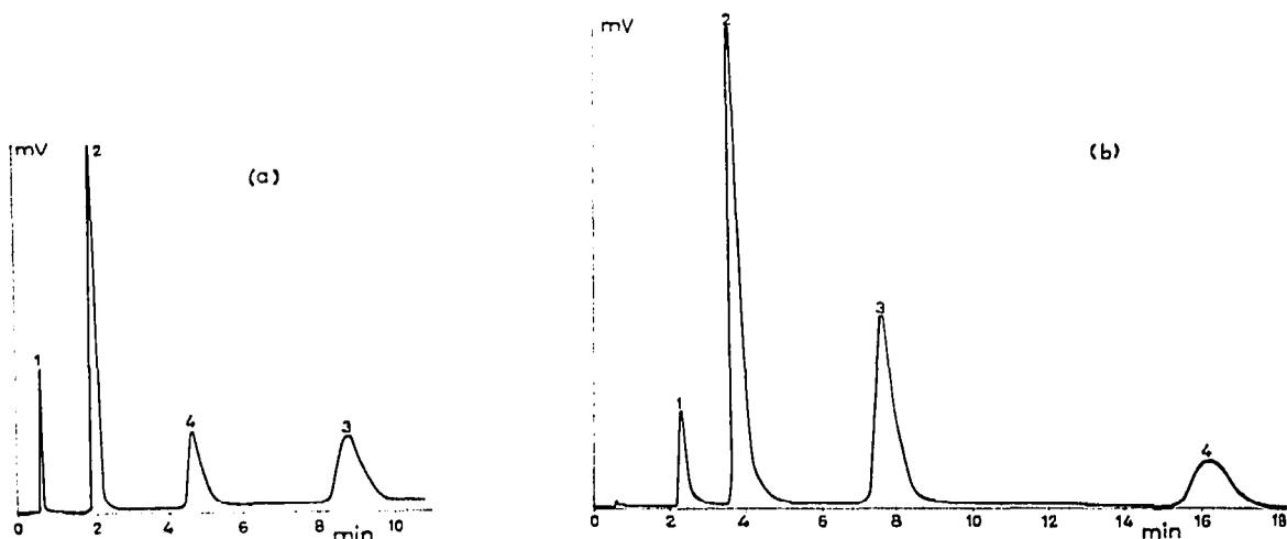
Fig. 4. Chromatograms of the system  $\text{H}_2\text{O}$  (1)– $\text{EtOH}$  (2)– $\text{EtOAc}$  (3)– $\text{AcOH}$  (4) on 2 m  $\times$  0.4 cm columns of (a) Porapak Q at 160° and (b) Porapak T at 180°. Carrier gas (hydrogen) flow-rate, 150 ml/min.
