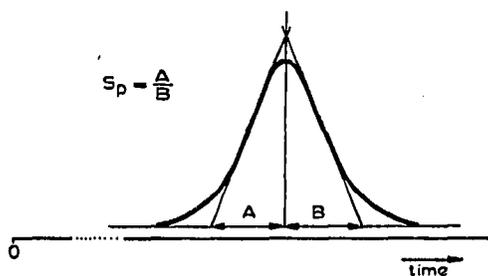
Fig. 3. Definition of  $S_p$  according to Fuchs<sup>20</sup>.
